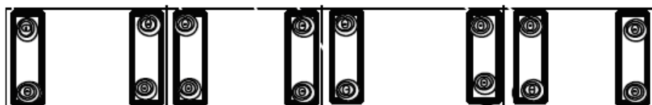
Earthquake Heavy Anchoring (showing placement of earthquake plates on framework base plate) .
